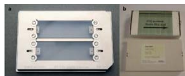
Fig. 1: MTP Slide Adapter II (a) and Glass Slides for MALDI imaging (b).
