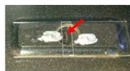
Fig. 3: Positioning of the CoverSlip on the glass slide.
